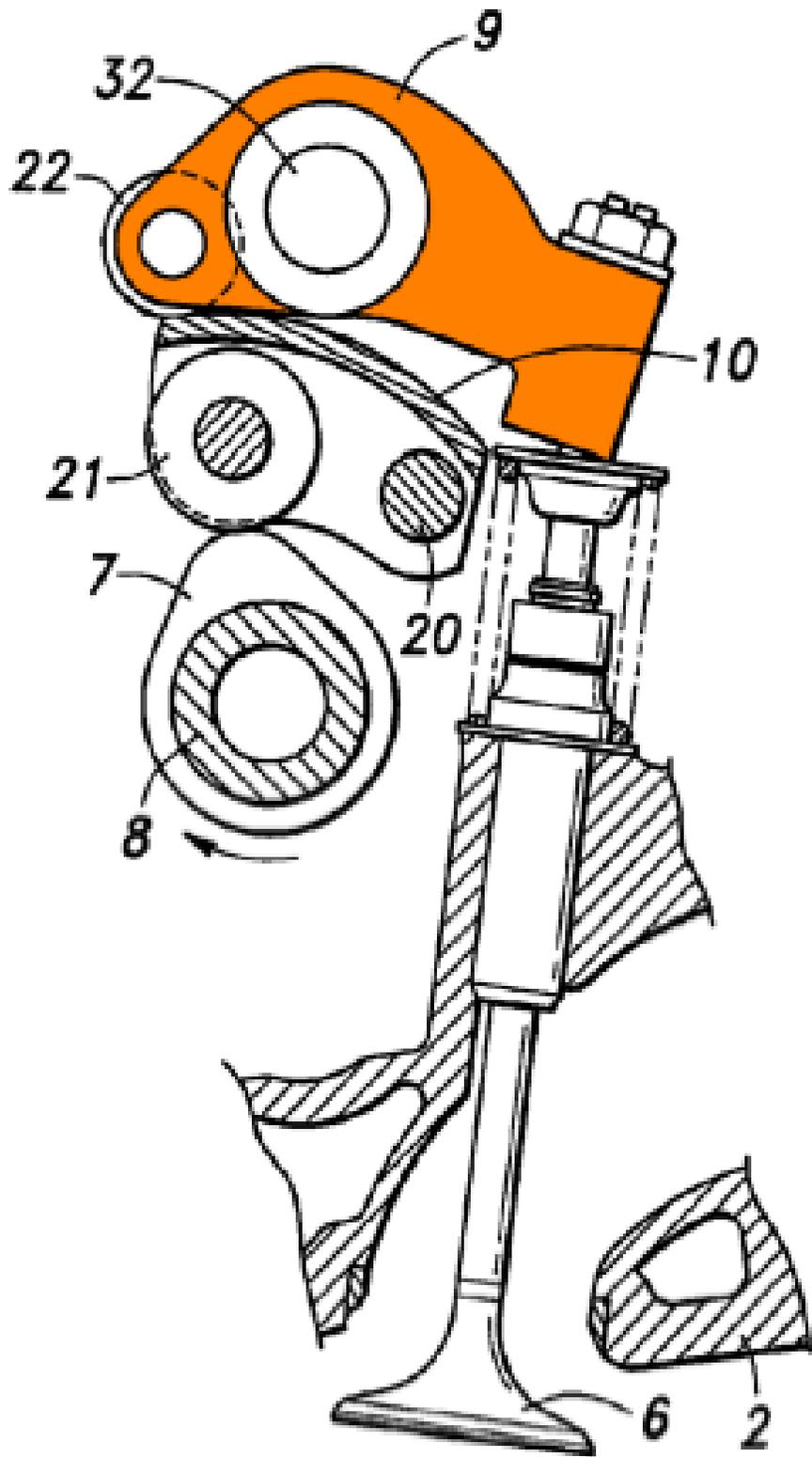
The cam, rocker arm and poppet valve. The rocker arm
