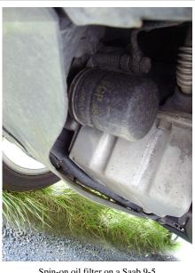
Spin-on oil filter on a Saab 9-5
