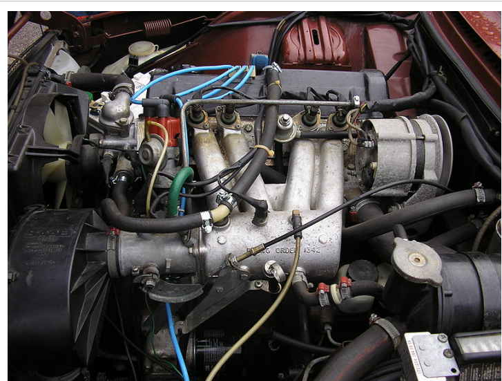
Saab B engine, "firing order 1342" marked on inlet manifold. #1 is towards the firewall (right side of picture).
