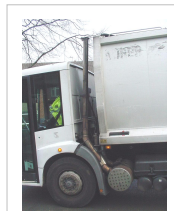
Waste collection vehicle's diesel exhaust pipe
