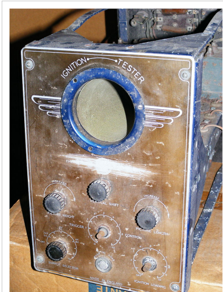
Igniscope ignition tester, with display tube and outer case missing.
