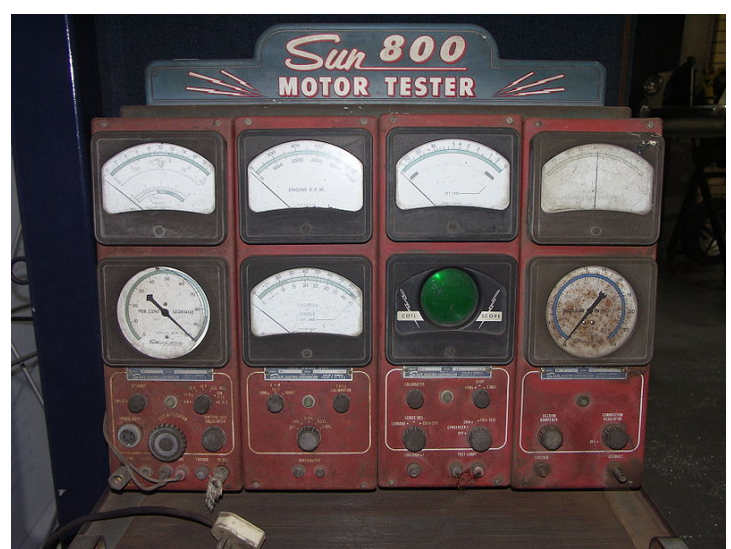
Vintage engine testing equipment that can test ignition timing, ignition dwell, manifold vacuum and exhaust emissions
