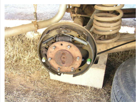
A drum brake with the drum removed as used on the rear wheel of a car or truck. Note that in this installation, a cable-operated parking brake uses the service shoes.
