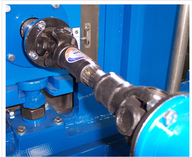
Drive shaft with universal joints at each end and a spline in the center
