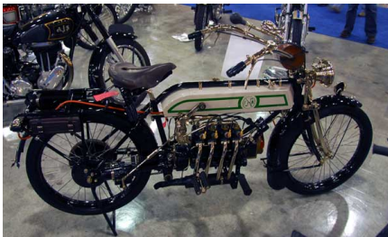
A 1913 FN (Fabrique Nationale), Belgium, 4cylinders and shaft drive
