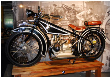
A 1923 BMW R32, with a shaft-drive, boxer twin engine
