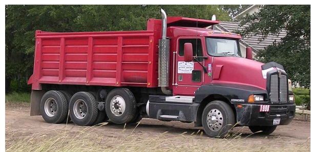
This dump truck has an airlift pusher axle, shown in the raised position.
