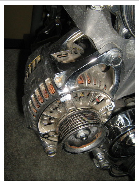
Alternator mounted in lower right front of an automobile engine with a serpentine belt pulley.
